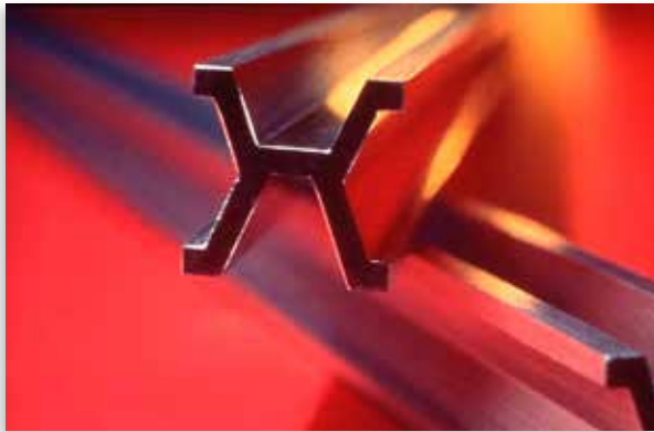
Figure 1.19 An original platinum bar in Paris, France showed the official length of a meter. 24
